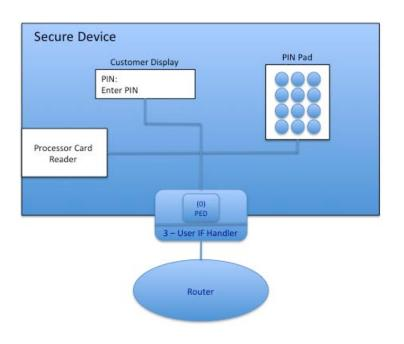
Figure 18: Secure Cryptographic Device
